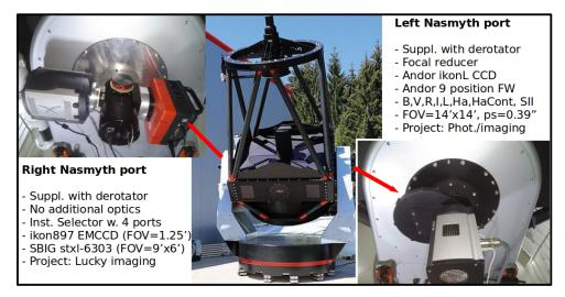
Figure 1: The 1.4m telescope (middle) and the two ports with image-derotator.
