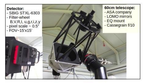
Figure 2: The 60cm telescope.
