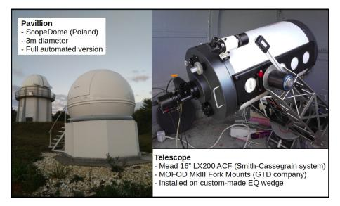
Figure 3: The 40 cm telescope.
